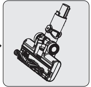
Fix the roller back to its place by pushing.
