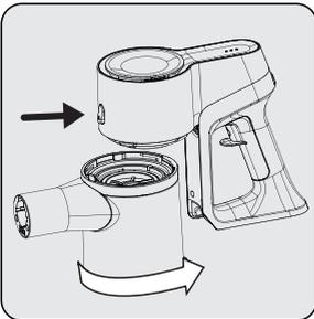
Fix the connector of dustbin to the holes on the body, then fix the dustbin by turning counter-clockwise until you hear the click sound.
