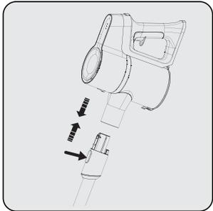
Push the tube (10) in the direction of arrow towards the body by pushing on the tube release button (6).
