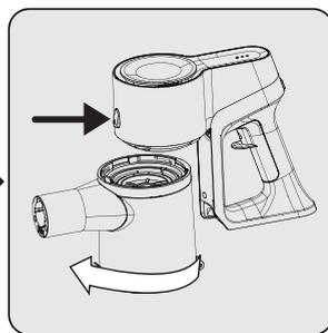
For a detailed cleaning of filters, remove the dust container by turning it clockwise.
