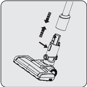
Press the electric turbo brush release button (11) on the electric turbo brush (12) and push it in the direction of arrow towards the tube.
