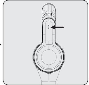
Flashing of the charge indicator LEDs (1) in white colour indicates that the appliance is being charged.
