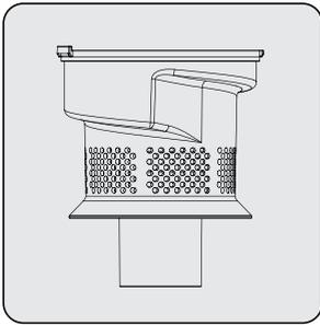
Attach EPA E10 filter to the plastic filter back.
