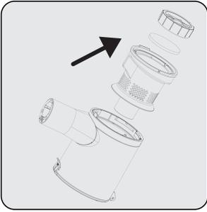
Pull EPA E10 and plastic filter holding ring from the EPA E10 handle.
