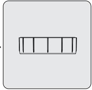
Remove the dust on the EPA E10 filter by tapping it on a hard surface such as a waste bin or by using a brush.
